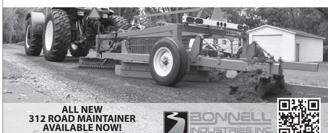
The Bonnell Road Drag repairs water damaged gravel roads 2.5 times faster than a motor grader, costs 90% less and saves you 50% on fuel costs. Save the wear and tear on your motor grader and use it to make roads, not repair them.
